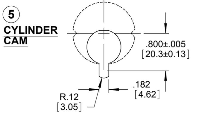
1830 SERIES LOCKS ARE OPERABLE BY ANY STANDARD 1 5/32" (29.3) DIA. MORTISE CYLINDER WITH SPECIAL "MS" CAM DIMENSIONED AS ABOVE. CYLINDERS WITH "MS" CAMS CAN BE READILY OBTAINED FROM MOST CYLINDER MANUFACTURERS.
