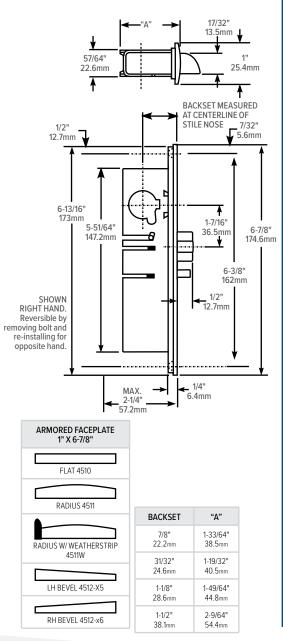
Stile Preparation Identical to MS1850S Series (Also see prep for 4590 Paddle) BACKSET STILE & . 1-19/32 40.5m 6-57/64" \_\_\_1-1/4"DIA. 31.8mm 175mm 6-3/8" 162mm TAP 10-32 2 PLACES 0 5/32" R TYP. 4mm 1-1/64" 25.8mm
