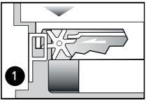
2. When push bar is depressed, the deadlocking slide moves back, allowing the door to unlock from the strike. This unique interlock provides solid security and prevents jamb spreading.
