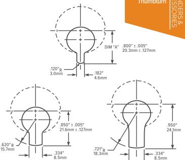
DIMENSIONS OF CAM TO OPERATE: 4070 SERIES DEADBOLT This cam available from above cylinder manufacturers on special order DIMENSIONS OF CAM TO OPERATE: 2331 DEADBOLT This cam available from all cylinder manufacturers (standard cam)
