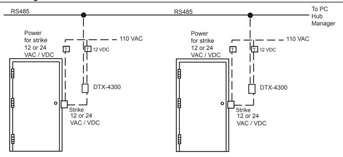
The Access Control System located at the door, acts as the reader and the controller. The wire connections are made at each door.
