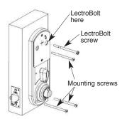
**Warning**: If using a power drill, please be careful not to over-tighten as this could cause damage to the mounting screws and threads.
