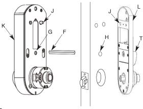
Ensure the red collar (J) is seated into its mounting hole. Carefully push the inside housing (L) flush against the door.
