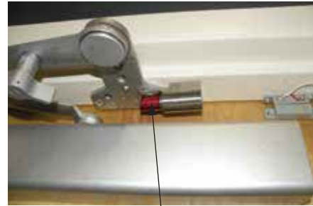
NOTE: PLUNGER HIGHLIGHTED TO ENHANCE THE CUSHIONING FEATURE.
