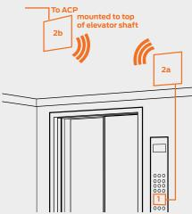
The ECK400 wireless elevator kit is ideal for retrofit applications, it eliminates the need to run traveling cables inside the elevator shaft. The reader is connected to the WRI400 on top of the cab. The WRI400 communicates over 900 MHz to the PIM400 on top of the shaft. The PIM400 is wired back to the ACP for real time monitoring.
