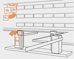
The GCK400 wireless gate kit is ideal for upgrading to real time access control on garage and parking lot entries. The GCK400 kit features open architecture devices and is compatible with popular Wiegand and Clock & Data format readers.
