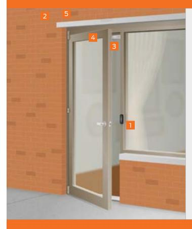
The CT5000 is an offline single door controller that can be used to provide the convenience of access control to openings that do not require real-time monitoring. An audit trail can provide a record of who requested access. It can work with a variety of readers, as well as interface with peripheral devices such as automatic operators, electric strikes, and electromagnetic locks.
