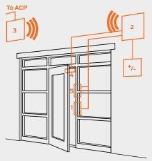
The WRI400 wireless reader interface is a networked access point controller designed to provide wireless connectivity to traditional electronic access control components, including standard Wiegand readers, door position, tamper, and request to exit switches.
