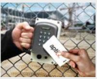
The WPR400 can validate credentials in real time when in range of the PIM400-TD2, which is connected to the access control panel. The WPR400 is capable of operating in cache mode, and when enabled, it keeps a local database of valid access grants. Upon moving the WPR400 to a location that is out of range the local database can be used to verify up to the last valid 1,000 users.
