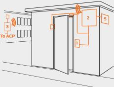
The WRI400 has a communication range of up to 1,000 ft. with clear line of sight. Remote antennas can be used to increase the range when needed. The WRI400 eliminates the need to dig a trench to the storage shed, saving time and money associated with equipment rental and running wires under ground.
