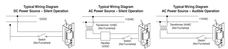
Typical Wiring Diagram for Electrified L-Series Locks
