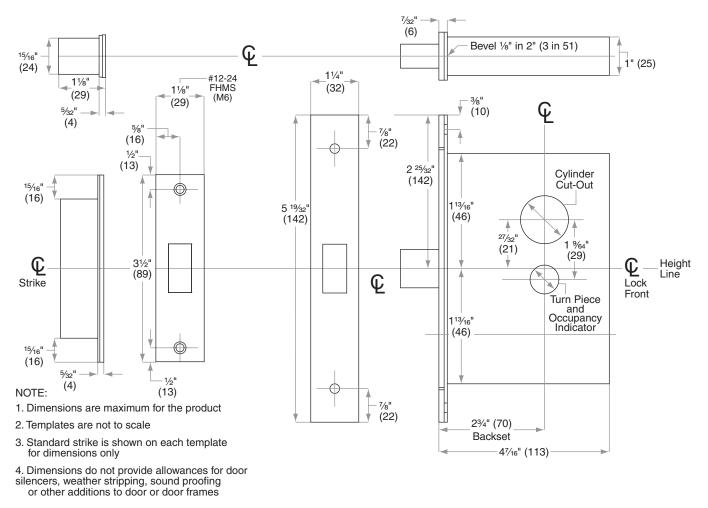
ANSI Standards: L400-Series locks meet all requirements for installations in doors and frames prepared in accordance with ANSI specifications A156.13, 2010
